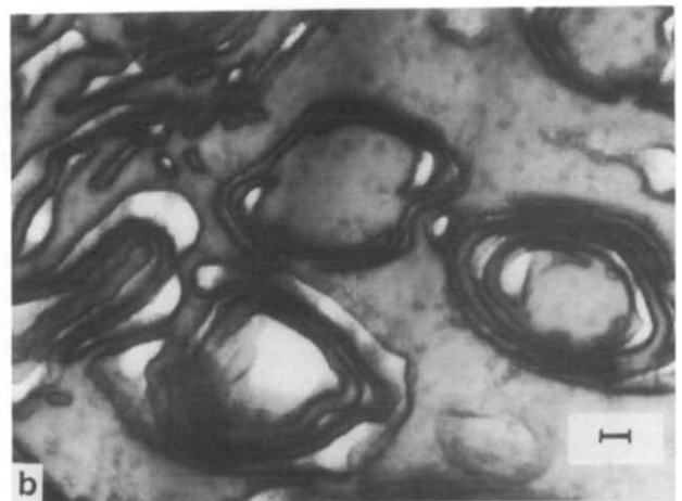
Figure 8 PPO/SBMA blends with 50 wt% SBMA obtained by method IV and stained with RuO 4 . Scale bars 0.1 μm
